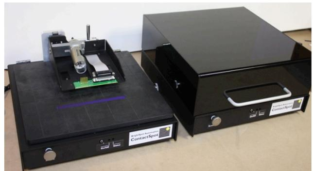
Fig. 1. *ContactSpot* tools for measuring contact resistivity
