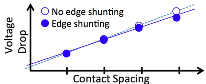
Fig. 6. Rollover effect in the TLM method leading to an overestimation of the y-intercept value
